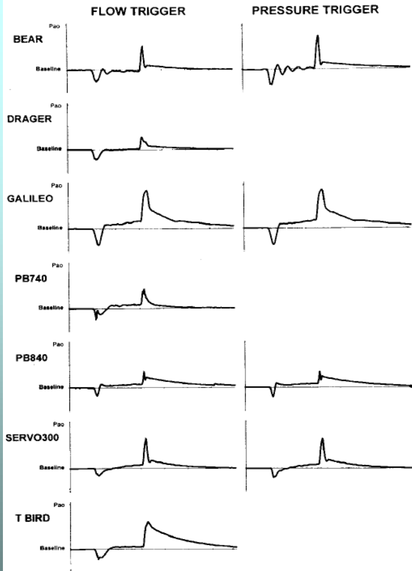
Fig. 3. Airway pressure versus time waveforms for all ventilators evaluated at 80 l/min peak flow. Pao = airway opening pressure.
